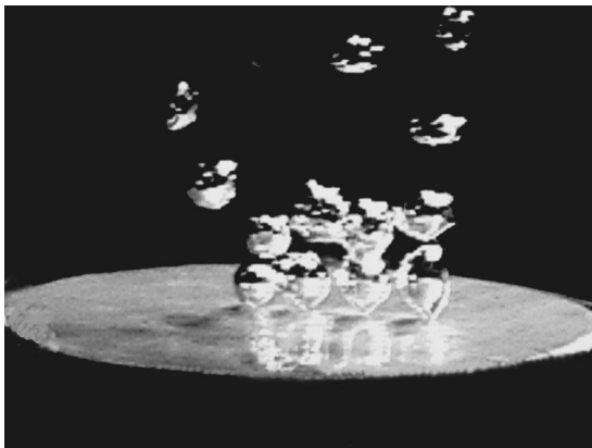
Fig. 2. Four active nucleation sites, arranged in a line.
